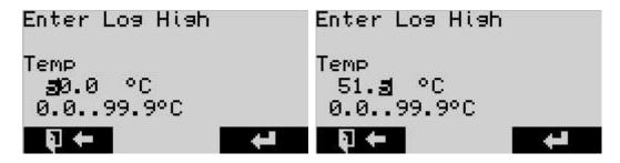
Change the value with the keys  $\uparrow$  or  $\checkmark$ , with **Enter** a digit is moved to the right. After entering the value, exit the mask with **Enter**.
