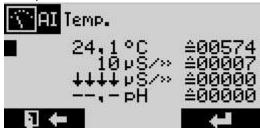
The input to be calibrated is selected with the aid of the  $\uparrow/\Psi$ -keys and branched to the following calibration mask. Here, the current measured value as well as the lower and upper calibration point are displayed as logical as well as converter raw value.
